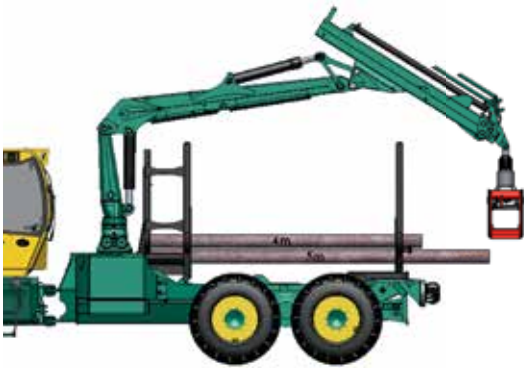
Variable last stanchion in "Medium" position
