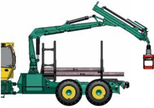
Variable last stanchion in "Short" position
