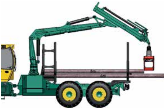
Variable last stanchion in "Long" position
