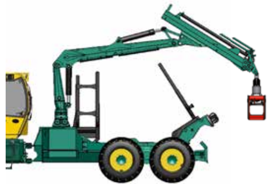
Skidding by rope possible without demounting the rung
