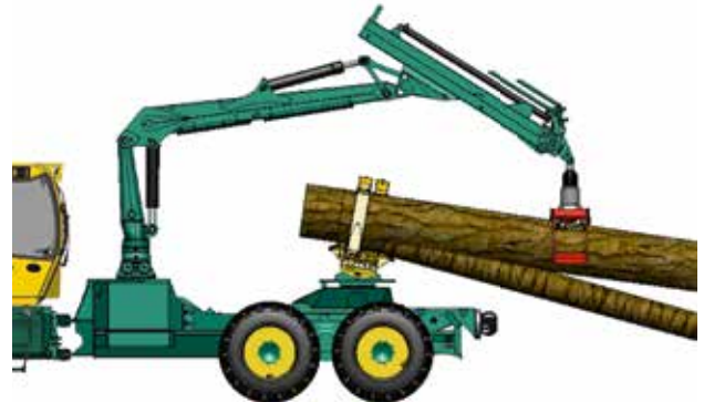
Skidding of long timber by quick-changeable clam-bunk
