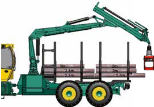
Quick changeable "Twin-rung" for 2 x 2 or 2 x 2,5 m logs (not at 805F version "short")
