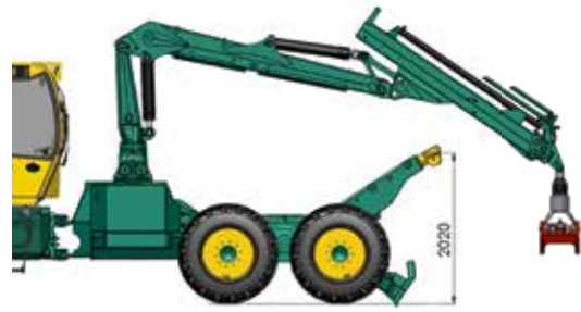
Height-adjustable rope-guides up to 2 m
