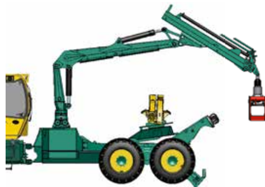
Skidding by rope possible without demounting the clam-bunk
