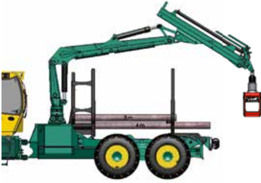
Variable last rung at position "short"
